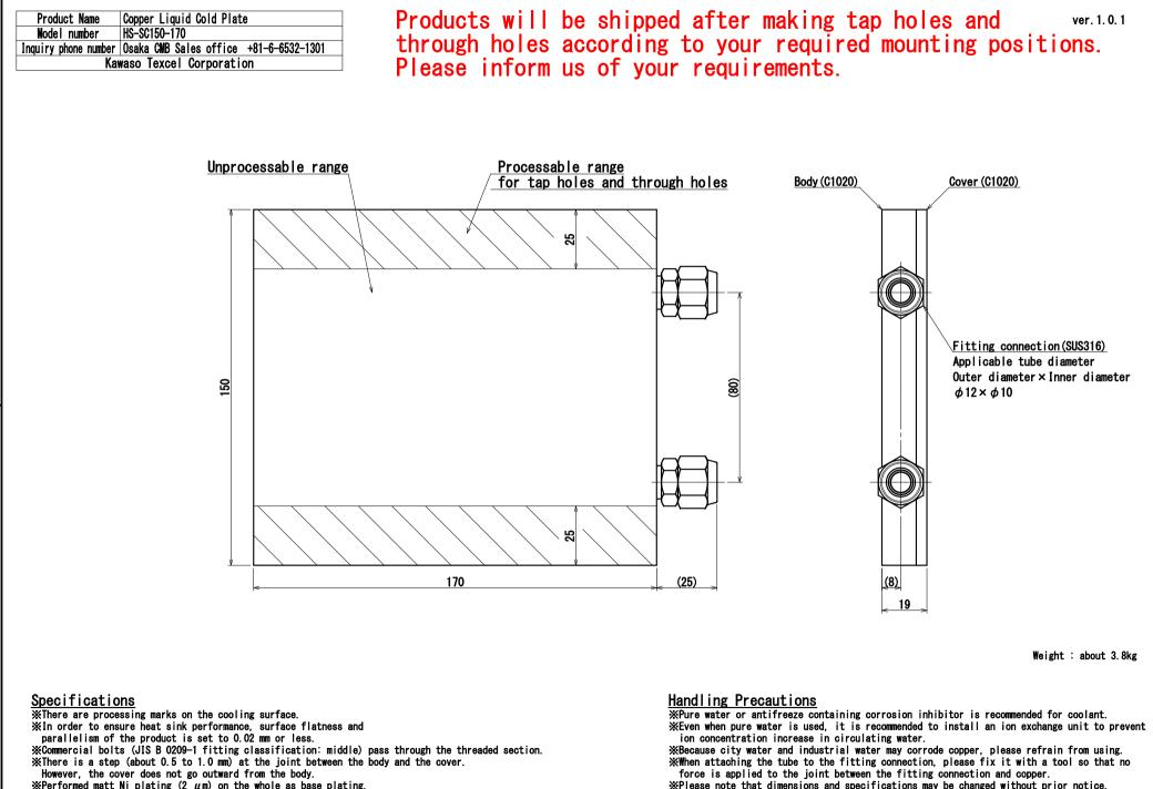
When machining inside the tapped holes, inside the holes may be non-plated.
